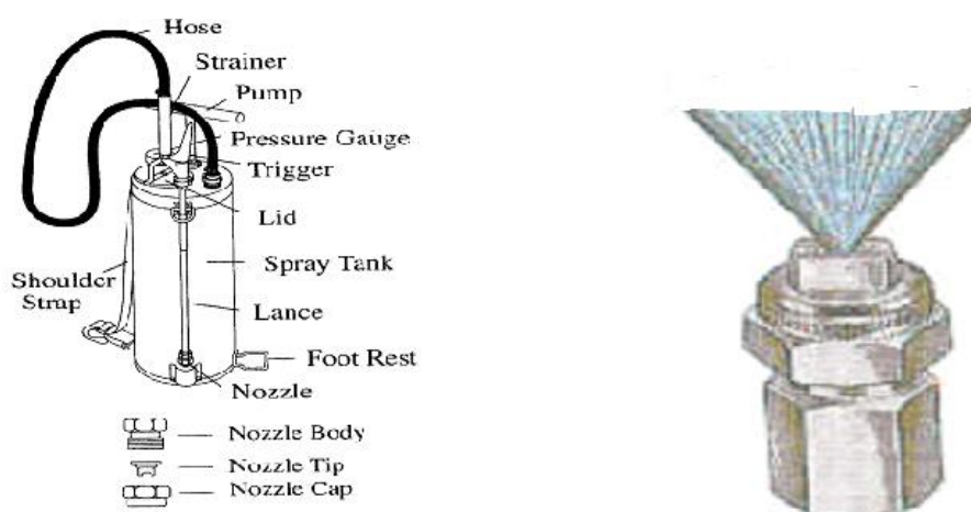
Fig.3.4 Spray can (left) and the fan shape discharge (right) of T-Jet 8002 nozzle tip.
